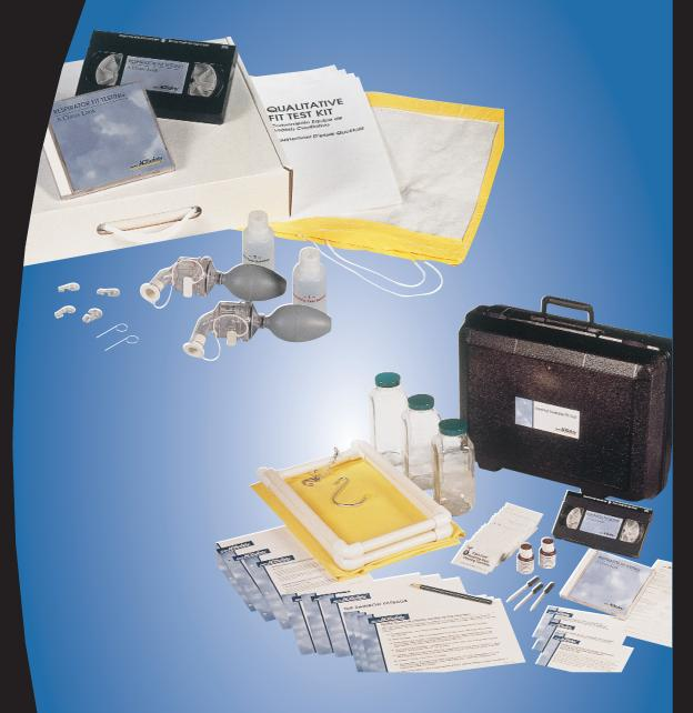
Convenient qualitative fit testing kits and quantitative fit test probes and adapters to make fittesting as easy as possible. All qualitative kits include complimentary instructional video and CD-ROM on how to fit test. The quantitative accessories make for quick conversion of an AOSafety® air purifying or airline respirator to fit test mode for those workers who want to be tested in their own masks.
